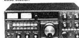
IC 271 — Icom's v.h.f. multimode base station
