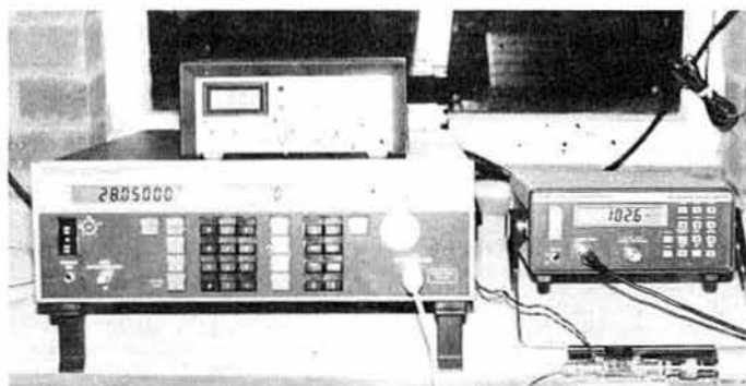
Photo 1. Testing the power meter; signal source (Marconi 2019 signal generator), power amplifier under test and power meter (Marconi 6960)
